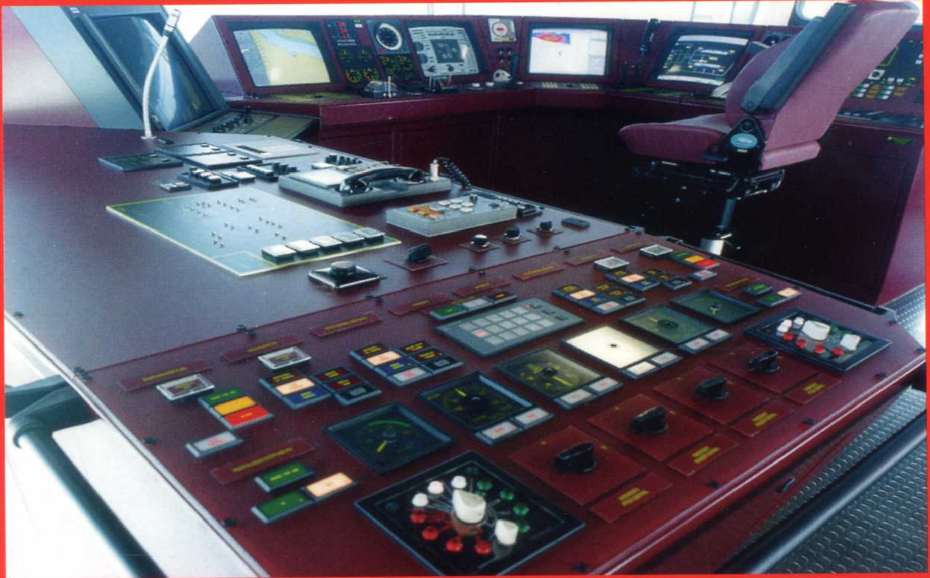
Fully integrated navigation bridge developed by IHC Systems
